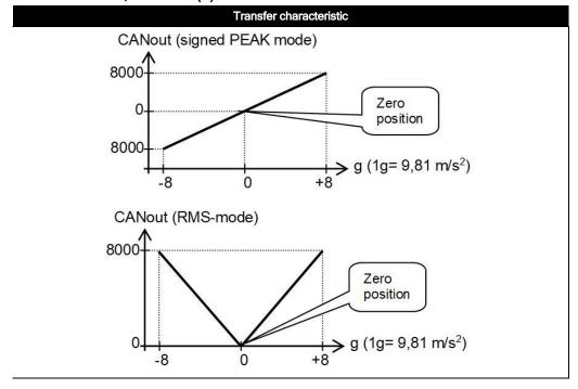
The default 0 g position is when the sensor is mounted horizontal or vertical and no acceleration is applied. The axis parallel to earth gravity will indicate 1 g, the two horizontal axes will indicate 0 g. The two horizontal axes can be zeroed within ±5° tilt (by the CAN object dictionary) to eliminate mounting offsets.
