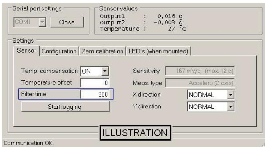
**To turn off the high pass filter, filter time must be zero (0)!**
