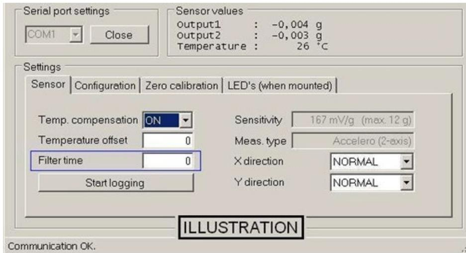
With the software program “ QGxx Configurator, the “ period time” of the high pas filter can be set. The program works with milliseconds (1/1000 of a second).
