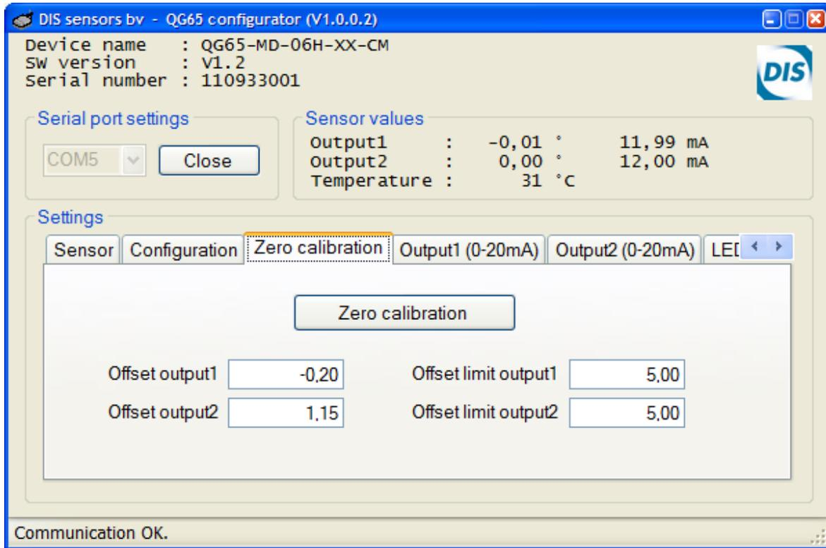
In this tab page the sensor can be calibrated.
