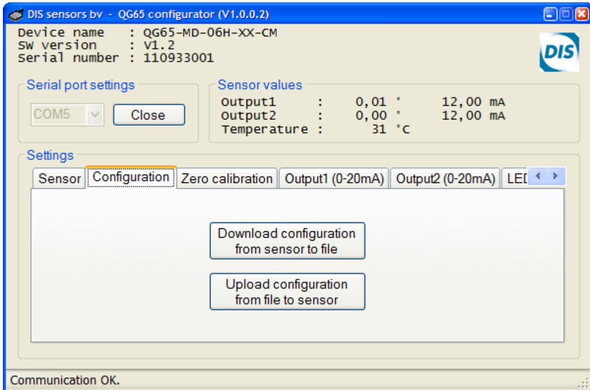
With this tab page the complete configuration of a sensor can be stored/restored to/from a file. The serial number of the sensor is stored in the file. During a restore it is checked that the serial number matched with the configuration file. If there is a mismatch the user can choose to upload the configuration to the sensor, although some settings in the sensor will not be overwritten.
